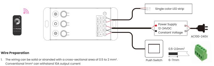
2. When wiring is installed, the terminals must be tightened. If they are not tightened, the contact point resistance will be too high and the terminals will easily burn due to heat when used at full load for a long time
