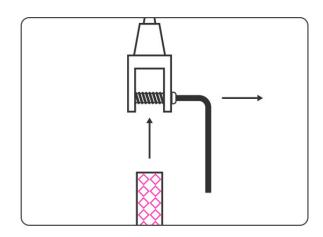
Unscrew the bolt from the clamp, insert acrylic backboard and align to hole
