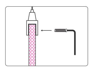
Thread bolt back into the clamp and tighten with allen key
