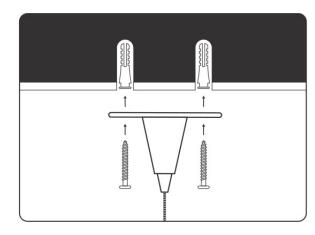
Use these measurements to screw the mounts into the ceiling
